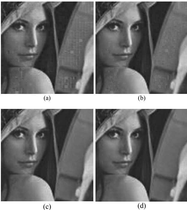
Fig. 8 Reconstructed Lena image using Entropy-based adaptive compression approach with 4 different compression methods (a) to (d) from Table II
